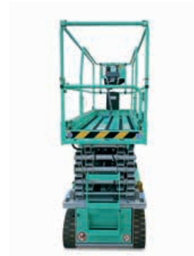
New design of the AWP and the scissor pack
